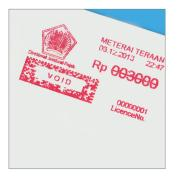
**Secure printing technology** The dual colour digital print protection (thermal-transfer) uses fluorescent ink against copying and blue ink for barcode verification via scanning devices.
